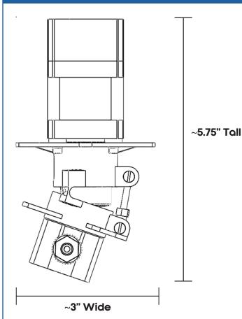
WETTED MATERIAL OPTIONS: Ceramic: Alumina, Zirconia Pump Housing: PVDF, ETFE, Polypropylene
